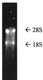
Fig. 1 Total RNA was analyzed by electrophoresis on 1% agarose gel
